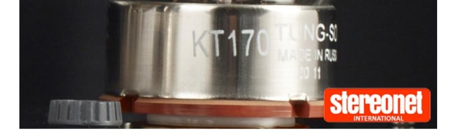
The KT-170 itself is a fairly large tube, not unlike a 300B in terms of size and appearance. The curvy domed shape is designed to maintain a high vacuum and improve heat dissipation. At its widest, the tube measures 6.5cm in diameter; Jadis provides a 3.5cm distance between each pair of tubes.
